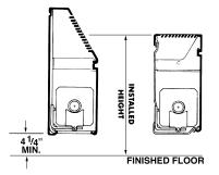
The **installed height** for enclosures is defined as the distance from the finished floor to the center of the outlet. Recommended height is based on a minimum mounting height for all covers and enclosures of 4½" from finished floor to bottom of front panel.
